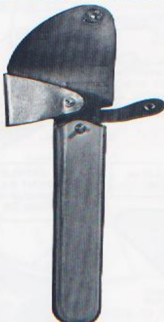
LEATHER CASE MADE FROM WOODEN FORM AT LEFT.
