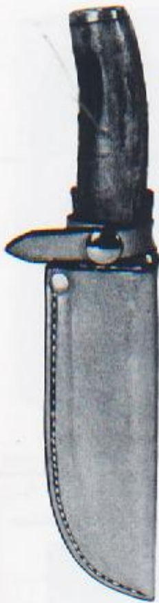
1 Fold and crease a piece of paper. Lay knife about 1/8" away from center fold, as shown. Pencil a mark under the guard, on both sides of blade. Draw a line, paralleling blade, 3/4" away... this will be the pattern cut-line.
