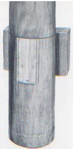
WOODEN MANDRIL SHOWING ADDITIONS CORRESPONDING TO THE CAMERA MEASUREMENTS
